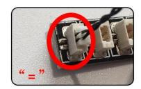
Connect the USB power cord to any port on the 4-Port Expansion Boards.
